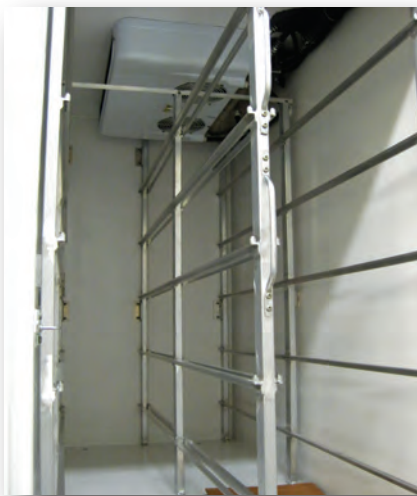
ES-300 evaporator mounted in a multi-temperature application.
