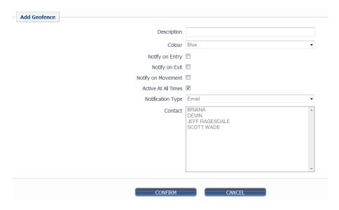
TIP: Ensure the vehicle you need to place a Geo Fence around is selected before confirming the Geo Fence. You can select multiple vehicles for a single Geo Fence
