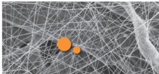
The fibers in the Thermo King filter media have submicron diameter and small interfiber spaces, which result in more contaminant being captured on the surface of the media and lower restriction.
