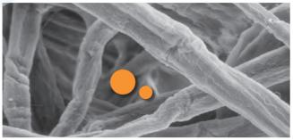
Cellulose fibers are larger and have larger spaces between the fibers, causing contaminant to load in the depth of the media and plug the airflow path; resulting in higher restriction and less capacity.
