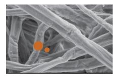
Cellulose fibers are larger and have larger spaces between the fibers, causing contaminant to load in the depth of the media and plug the airflow path; resulting in higher restriction and less capacity.
