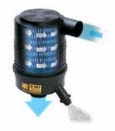
EMI-3000 air filters offer the greatest efficiency in air filtration for Thermo King equipment via the two-stage cyclonic action process. 75% of the particles are removed from the filter out the evacuation valve before they even reach the filter media. This allows only the Thermo King filter to reach maximum efficiency of 99.97%.
