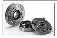
Clutch Assembly 2B, 24V Order Part #: P-50-01122-07 (Replaces Carrier #: 50-01122-07)
