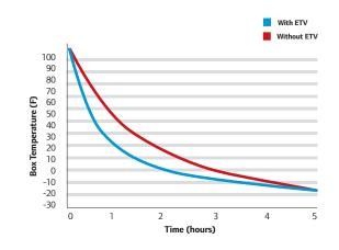
The Electronic Throttling Valve (ETV) on Thermo King trailer units protects fresh loads while saving you time and fuel. ETV also maximizes high ambient temperature operating performance, improving load safety in hot summer weather.
