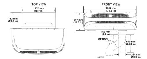
NOTE: The top of the unit to be mounted flush with the top of the cargo box when possible. The top of the evaporator to be positioned 25.4 mm (1.00 in.) below ceiling.
